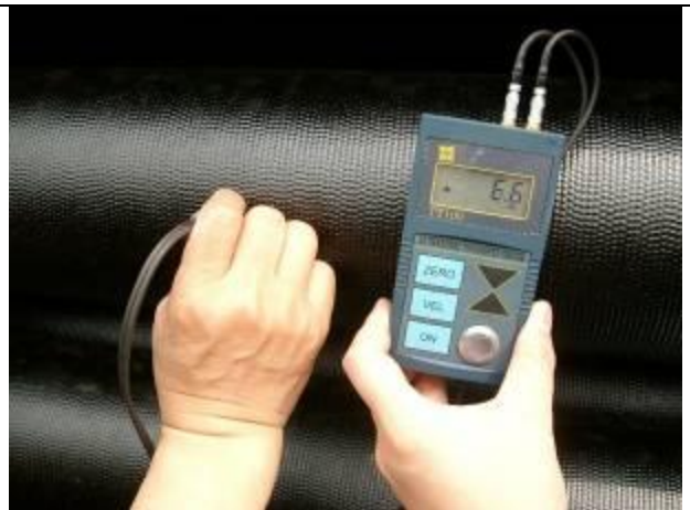
Wall thickness checked
