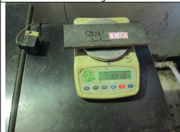
Witness zinc coating check
