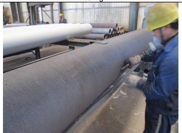
Witness zinc coating check
