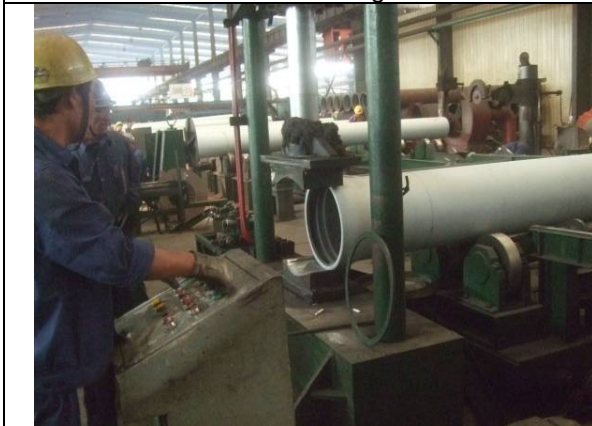
Socket check and adjusting
