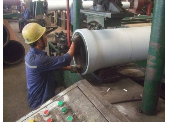
Socket check and adjusting
