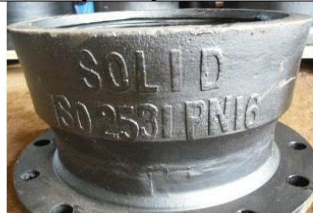
Mold marking on Socket Flange
