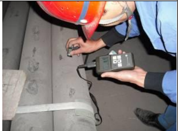
Wall thickness checking
