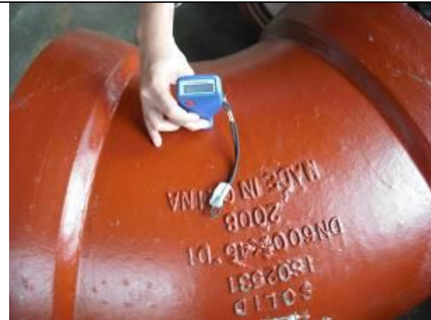
Bitumen layer thickness checking
